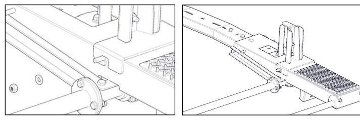
• If using an "Extension Ladder" put the Ladder Stop(I) at the same location on the Front & Rear Bow Assy.(A&B).
