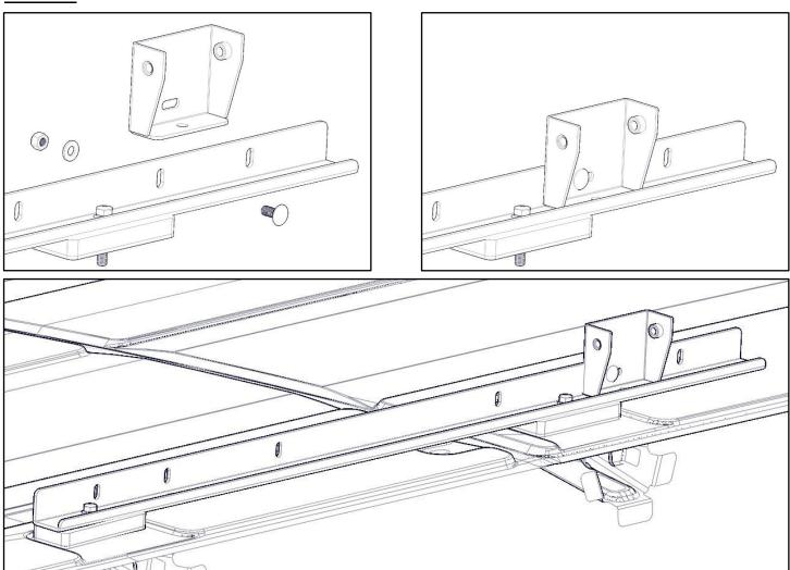
Notice the short feet are installed at the front.
