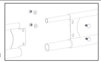
\*\*Be sure to apply sealant around tube connections\*\*
