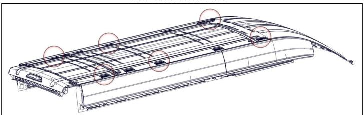
• Use the dimensions measured from the roof mount locations (X & Y) and coordinate onto the rack crossbars. Some slight adjustment will be available once rack is placed onto roof.
