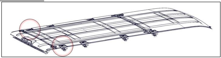
\*\* Place sealant around the exposed holes in the roof of the van under the rubber pads to ensure no water can leak into the cabin of the van. \*\*
