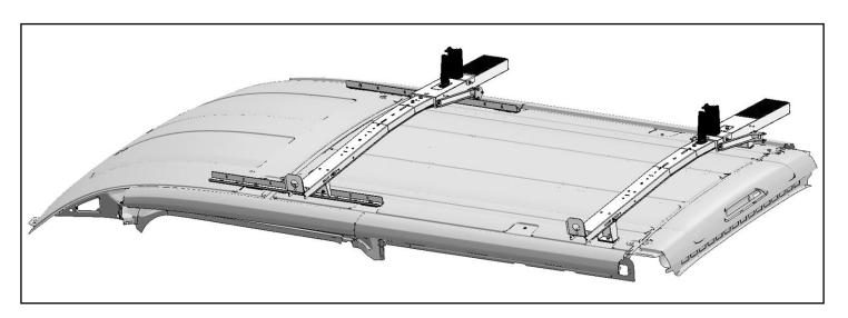
Step 3 - Torque Tube Installation
