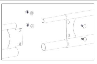
• Bolt using two 5/16 carriage bolts, two 5/16 flat washers and two 5/16 nyloc nuts. Repeat for a total of two rails assemblies.
