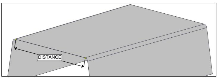
• Determine best mount locations on top of the shell and measure distance between the desired mounting locations.
