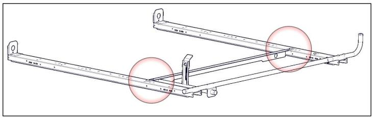
• Insert plastic bushings into the clamp and lock L bracket and the rotation bar plate installed in Step 4, with flange towards each other and to the inside as shown.
