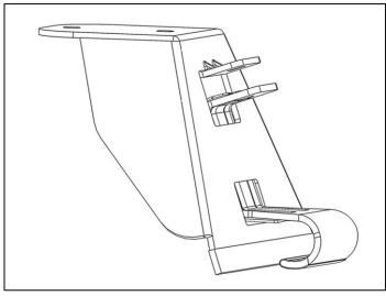
• LOOSELY bolt the gutter clamp to the gutter foot using a 5/16" x 1-1/4" carriage bolt, 5/16" flat washer, and 5/16" lock nut. DO NOT tighten.
