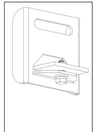
Slide an assembled load plate onto the middle of the crossbar with the load plate angled flanges facing outward. The slider plate should fit into the extrusion so the slider plate cannot rotate out of the extrusion.
