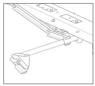
If installing on a High Roof Extended Transit, the Handle Extension (L) will be used. This extension goes inbetween the rear bow (B) and the actuator (F).
