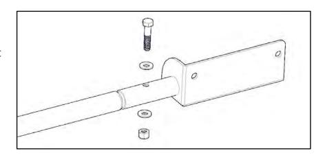
\*\*If installing on a High Roof Extended Transit, the support tube extension (L) will be used\*\*
