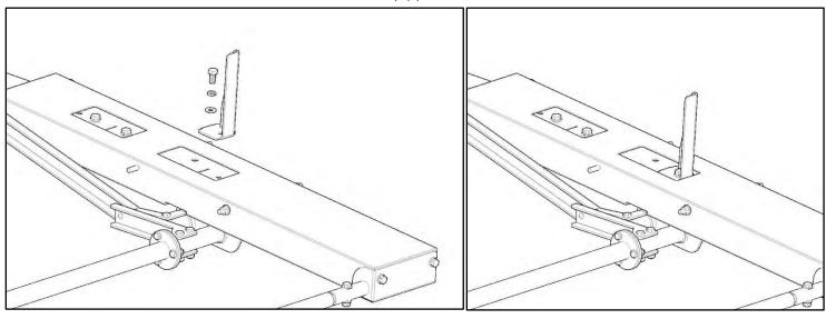
• Bolt Ladder Hook (H) to the lower position where the pem studs are installed. Use a .312 flat washer(6) and a.312 nyloc nut (9).
