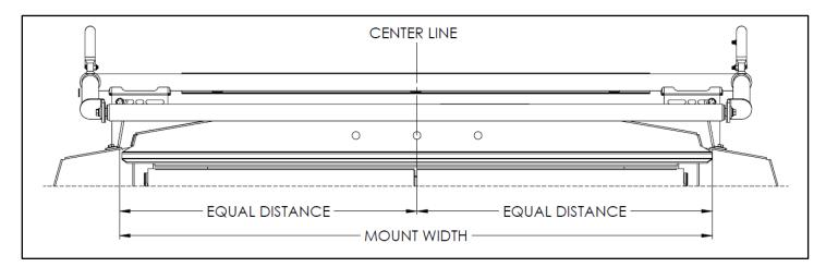
• Ensure the rear of the rack is far enough off the rear of the vehicle that when placing a ladder on the rack, the ladder does not hit the vehicle.
