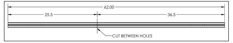
• The short rail is for the rear. The longer section is for the front.
