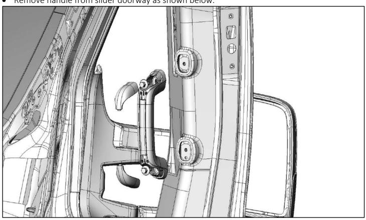
• Install handle mount (D) where handle was previously removed using M6 x 25mm HH (14), M6 lock washer (16) and a M6 split lock washer (15). SNUG TIGHTEN.
