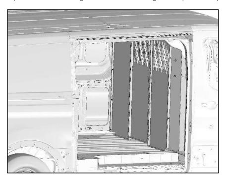
• Along the floor, at each plusnut, bolt through partition panels using 1/4" x 1.25" hex head (1), 1/4" lock washer (8) and a 1/4" flat washer (7). Insert nylon spacer (17) underneath partition if needed. SNUG TIGHTEN
