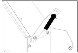
In the remaining locations along the wings, screw self tap bolts into van.
