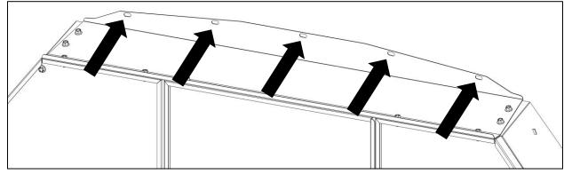
• Using 5/16" x 1" self tapping screws, install the corner brackets to the "B" pillar as shown.
