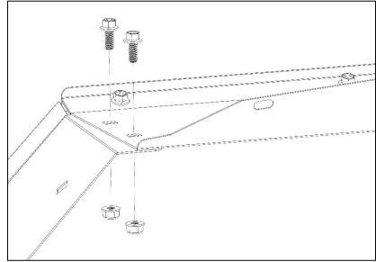
Using two 5/16" x .625" flanged bolts and two 5/16" flanged locknuts, bolt corner panel to side wing.
