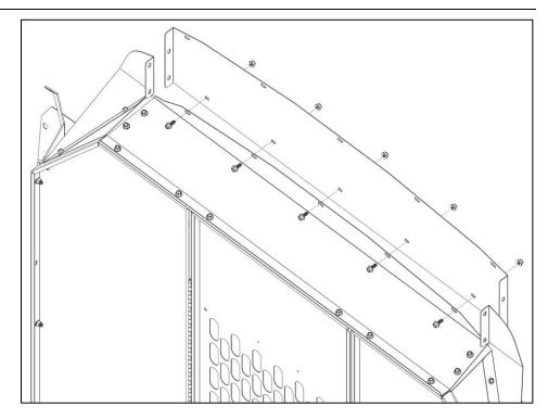
• Using two 1/4" x 5/8" flangd bolts and two 1/4" flanged locknuts, bolt each corner wing to corner panel.
