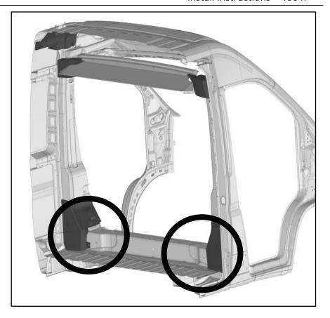
• Bolt bottom wing (B) to the 2 outside plus nuts (7) previously installed using 1/4" x 1" hex head bolts (4), 1/4" lock washers (5) and 1/4" flat washers (6).
