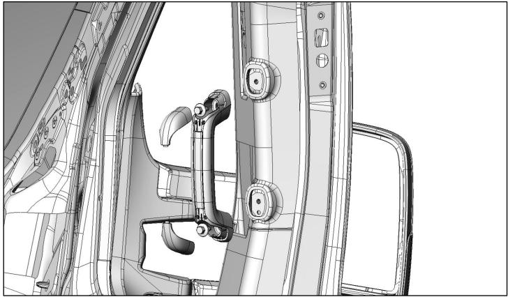
• Install handle mount (D) where handle was previously removed using M6 x 25mm HH (14), M6 lock washer (16) and a M6 split lock washer (15). SNUG TIGHTEN.
