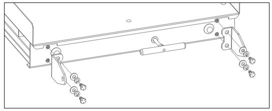
• Using two 3/8" x 1-1/2" button head screws, two 3/8" lock washers, and two 3/8" flat washers, install the pull handle assembly to the handle brackets. DO NOT overtighten.
