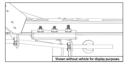
• Thread bungee cord through snap bushings on one side of ladder rack and then back through opposite side snap bushings.
