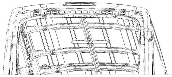
• If the rail assembly is too long, either mark or measure the length of horizontal rail that needs to be removed. The length of the uncut assembled rail assembly is 96".
