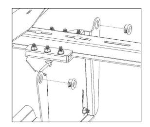
• Install 10-24 x 3/8" socket cap screw and 10-24 lock nut in hole at end of rail behind sliding bracket assembly.
