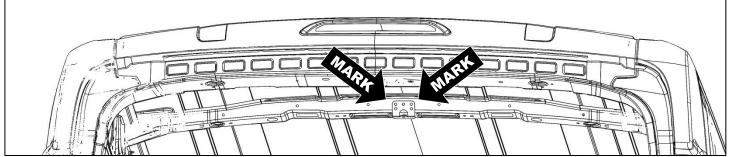
• Hold second mounting bracket against the center of forward roof support beam. Be sure the mounting bracket is level to the roof support beam. Mark mounting hole locations on the roof support beam.
