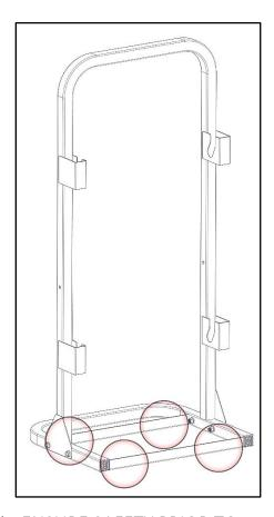
2. Use plus nuts. Mark location on floor, drill with a 25/64" bit. ENSURE SAFETY PRIOR TO DRILLING. Install plus nut into hole. Bolt cable reel holder to installed plus nuts using 1/4" x 1-1/4" hex head (5), 1/4" split lock washer (6) and  $\frac{1}{4}$ " flat washer (7). This is the strongest and recommended installation. TIGHTEN.
