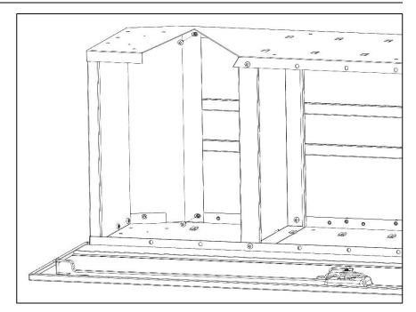
• Install two 1/4" x 3/8" one-way screws through the rear cover panel into the top rear shelf panel flanges.
