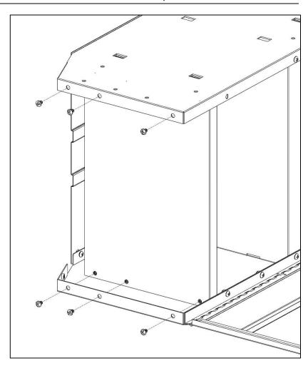
• Slide the rear cover panel inside the shelf-panel rear flanges and outside the top rear shelf-panel flanges.
