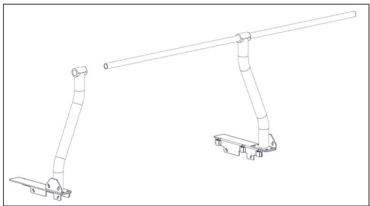
• Slide the crossbar through two roof rails (A or B).
