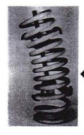
**NOTE** - Some General Motors and Ford vehicles have slightly curved coil spring assemblies. To preserve the curvature of the compressed spring, install the tool with short arms and long arms located on the same side of the spring as shown. Compress only enough to free the spring and provide clearance for removal from or installation into the spring seats.
