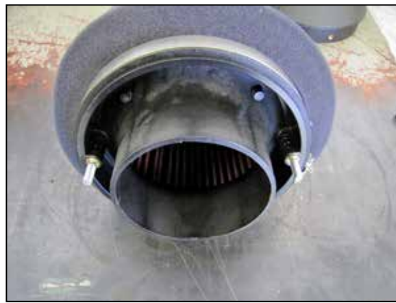
3. Install the two provided 6mm studs into the radius filter adapter as shown.
