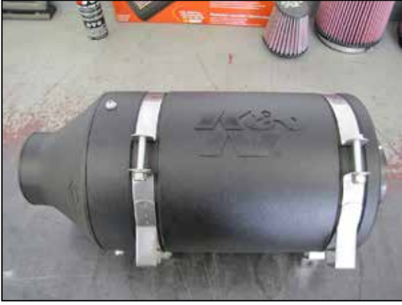
7. Install the saddle clamps onto the canister and secure with the provided hardware.
