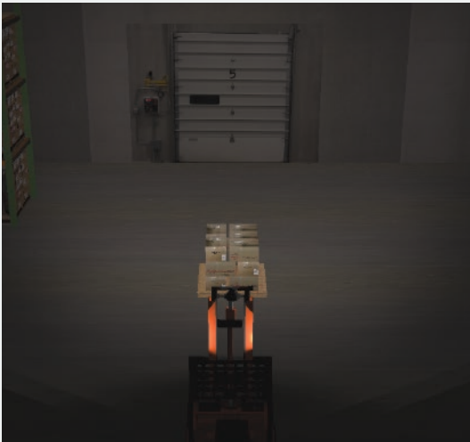
Traditional flood patterns create glare and lack intensity where it's needed the most
