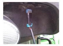
6. Attach LED lamp to combine, use previously installed 13mm hex head mounting bolts.
