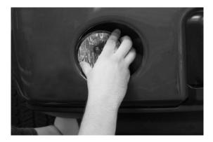
**5.** Orient the back of the mounting bucket so the word **"TOP"** is at the top. Insert the plastic nut into the square hole of the tab from the **BOTTOM**. It will snap into place.
