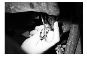
**3.** Facing the front of the vehicle, locate the mounting tab on the **RIGHT** side of the stock fog light. Use the flat blade screwdriver to depress the mounting tab until the post is released from the mounting tab.
