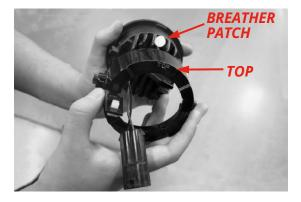
**9:** Take the light with the **"TOP"** text on top (when looking at the light from the back), and feed the wires through the hole in the shroud. Ensure that the **"SPEAKER"** logo is right-side up across the bottom of the front of the light. **Caution: If installed incorrectly, the light pattern will be upside-down** and will NOT be street legal.
