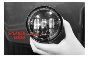
Caution: If the light does not pivot freely up and down, the installation was not done properly. Remove the light and start over from step 8 and verify that the mounting bucket has been properly attached.
