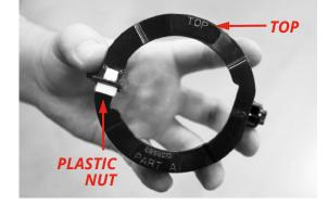
**6.** Holding the J.W. Speaker lights face-down, orient them so that the breather patch is at the **TOP** and the wiring is on the **LEFT**.
