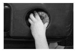
18. Reconnect the vehicle's battery. Turn on the lights to ensure that they are correctly installed and functioning. If they do not turn on, please check your electrical connections.
