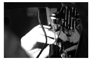
**13.** Reconnect the wire harness. **Optional:** The wire harness may be secured behind the mounting bucket with a zip tie (not included) to prevent accidental disconnection of the light.
