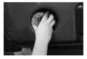
**5.** Holding the J.W. Speaker lights face-down, orient them so that the breather patch is at the **TOP** and the wiring is on the **LEFT**.
