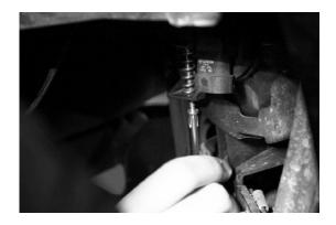
3A-2. Using one hand at the front and one at the back of the light, wiggle the stock fog light free from the shroud. Caution: If you depress the LEFT side first, the light will get stuck. Avoid applying excessive force as it may break off the mounting tab inside the shroud.
