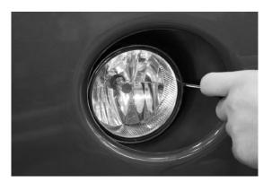
**12.** Using the #2 Phillips screwdriver or socket wrench, rotate the adjustment screw (clockwise to raise, counterclockwise to lower) on the rear of the lamp to aim the light like the existing fog light. **NOTE: The horizon (cut-off from light to dark) of the two lamps must align.**
