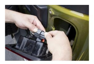
**4.** Feed the provided screws through the top of the resistor and attached the provided nuts by hand.
