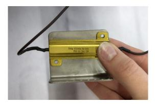
**5.** Secure the nut on the back of the resistor mounting bracket with a pair of pliers OR adjustable wrench, then tighten both screws with a Phillips screwdriver.
