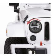
**10.** Re-attach the retaining ring. Align all 4 tabs on the ring with the screw holes. It will only fit in one orientation. Install 4 screws from step 5 using the T15 Torx driver.
