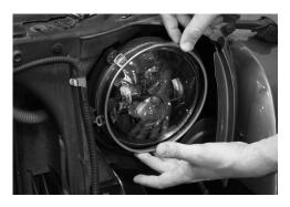
**7.** Unplug the existing headlight and turn signal. **NOTE:** On newer models there is (1) a red button on the plug that must be pushed up, and (2) a button that must be pressed and held to unplug the existing lamp.
