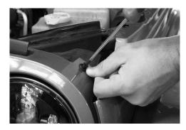
**2.** Carefully remove the 6 fasteners by prying them up at the base using a flat blade screw driver. Save the 6 fasteners.
