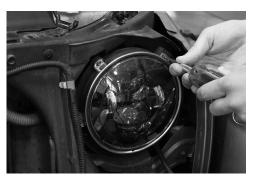
**6.** Remove the retaining ring and headlight from the mounting ring. Box" are present and complete.
