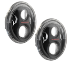
Part Number 0554563 12V ECE LHT LED High & Low Beam Headlights with FP, DRL, & Black Bezel - 2 Light Kit
