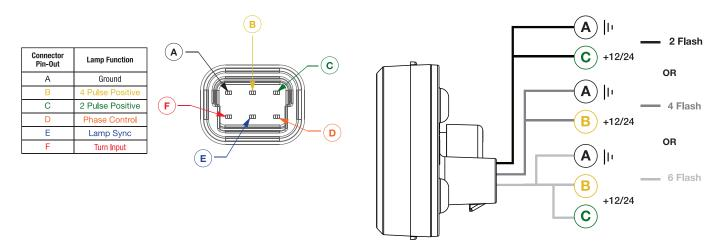
2. By connecting the Phase Control Wire (D) to power on one lamp and ground on the other lamp it causes an alternating pattern. To set the lights to flash at the same rate link the Phase Control Wire (D) to ground on all lights.
