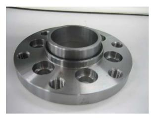
This is how it should look when done, the sleeve adapter portion will protrude thru the center hole of the flexplate towards the converter side, the I.D. of this will accept the 1.702 OD of any standard GM converter pilot. This is ready to be installed on the flexplate.
