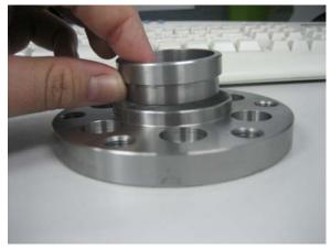
This is the 80015 adapter, notice the slight taper on the OD, it should taper down to 1.838"-1.842". This will accept the small OD of the 80002-1 sleeve adapter.
