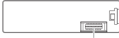
Connector (on the reverse side of the faceplate)
