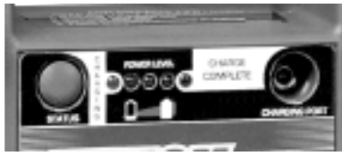
Figure 2. Test Button, Charging, Power Levels and Charge Complete LEDs
