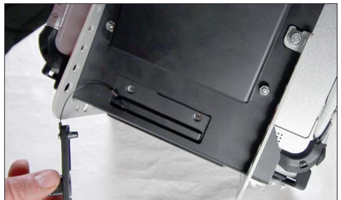
Secure connector to rear of iKey Keyboard.
