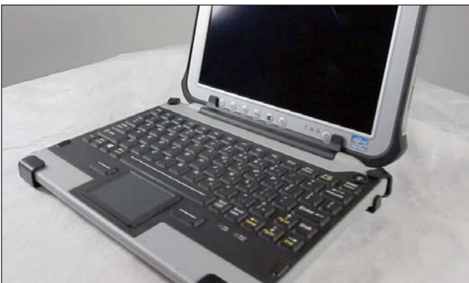
Place Toughpad FZ-G1 onto iKey Keyboard and Mounting Station.
