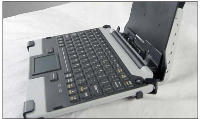
Position iKey Keyboard hinge/connection point to match mounting station angle.
