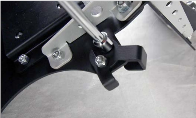
Loosen locknuts on back of Mounting Station. Remove brackets.
