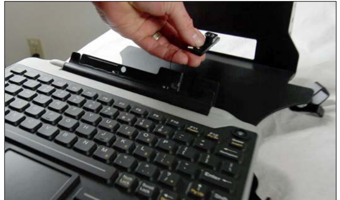
Place your iKey Keyboard into Mounting Station, making sure locking connector is passed through opening.
