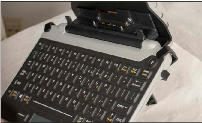
Replace brackets and tighten locknuts.
