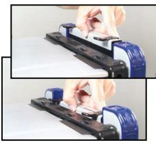
8.) Make any adjustments needed to the Rear Tabs to allow access to any data ports which may have been blocked by the original clamp positions. Loosen the Rear Tab screws (but do not remove) as shown in the image below. Adjust the Rear Tab as needed by sliding side to side in the adjustment tracks. Re-tighten Rear Tab Adjustment Screws.
