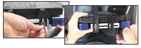
4.2) Using the New Side Clamps, install one New Side Clamp into each the slots that the Original Side Clamps were in previously. Tighten the screws. Ensure that all Side Clamps slide over the top edge of your laptop before moving to step 5.
