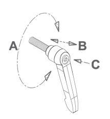
**NOTE:** Insert the ratchet handle through the unthreaded side of the articulated swing arm and tighten.
