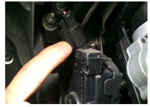
Step 2: Unplug the wiring harness from the pedal position sensor.
