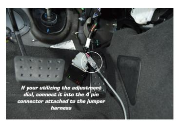
**Step 7:** Tuck the JMS module the opening above the TPS harness. Use the provided zip ties to ensure it doesn't fall out of place.
