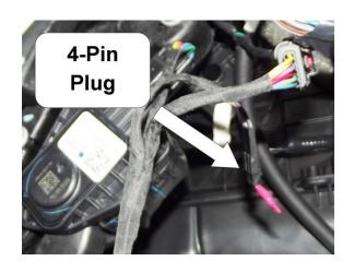
**Optional Control Accessory:** The optional single pedal knob (P/N BX-6999-SINGLE) is designed to plug in to the 4-pin connector and over-ride the preconfigured throttle response settings. With this option, you have ultimate control over the sensitivity with a range of 0% increase to the 100% maximum increase, based on the position of the control knob.
