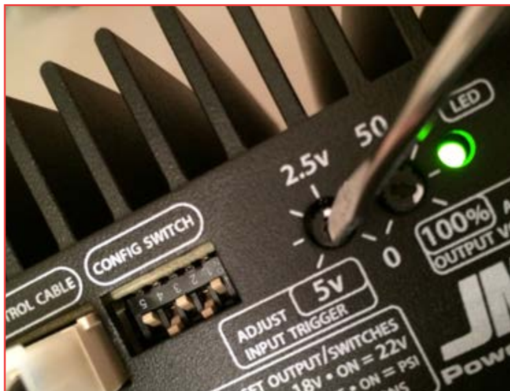
Dip SW 1 - Turn OFF to Save LED Twinkles when saving the front panel settings
