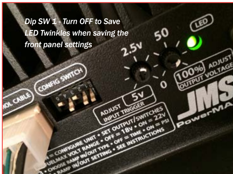
Accelerator Pedal Voltage Boosting occurs at just above 1/2 pedal. Green LED blinks when boosting
