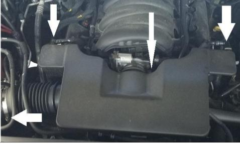
Remove stock PCV hose from PCV valve and intake manifold. Depress grey tabs to release hose, feed house out towards the front of the engine.
