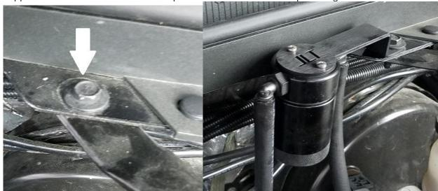
Run the short hose to the intake manifold, the connections will "click" once fully seated. Run the longer hose to the PCV valve, route under wiring harness and EVAP Solenoid.
