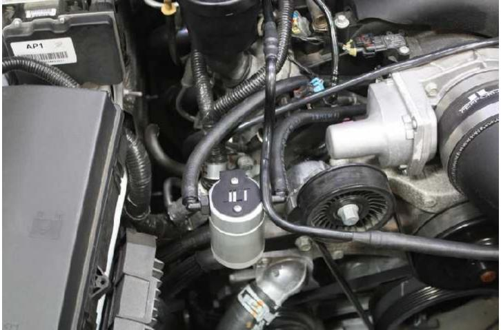
To properly clean the filter in the Oil Separator, spray any degreaser or solvent through it and let it air dry. Clean it every 10,000 miles. Thanks for the business.
