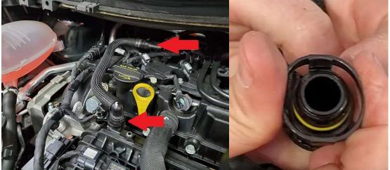
Now you will need to remove the fittings from the OEM hose you just removed. There are two ways to do this. **Option #1** You will need to heat up the hose near the fitting with a heat gun or lighter. We recommend wearing gloves or wrapped a rag around the fitting when attempting to remove them. **Option #2** Using your utility knife/razor blade cut the hose near the fitting to split it vertically to remove fittings, softening the hose with heat may help this process.
