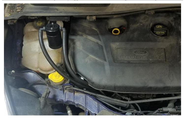
To properly clean the filter in the Oil Separator, spray any degreaser or solvent through it and let it air dry. Clean it every 10,000 miles. Thanks for the business.
