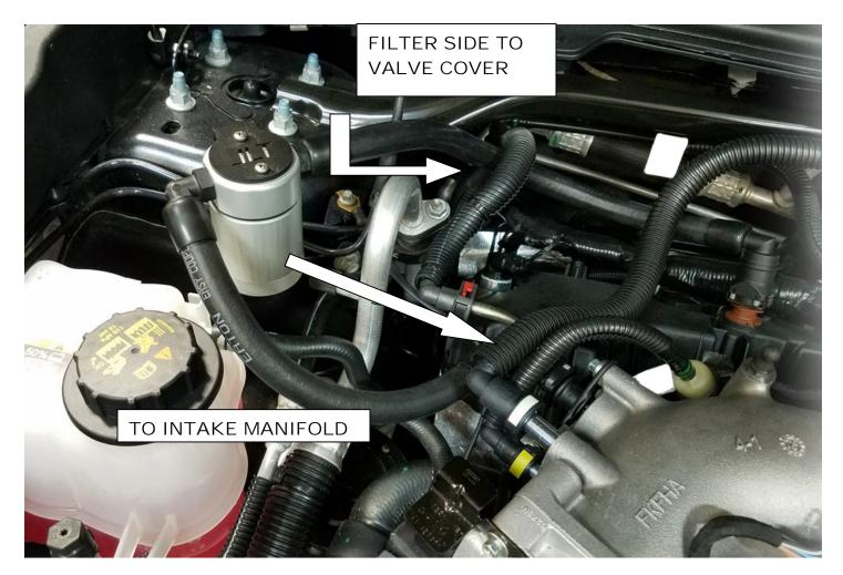
To properly clean the filter in the Oil Separator, remove it and spray any degreaser or solvent through it and let it air dry. Clean it every 10,000 miles. Thanks for the business.
