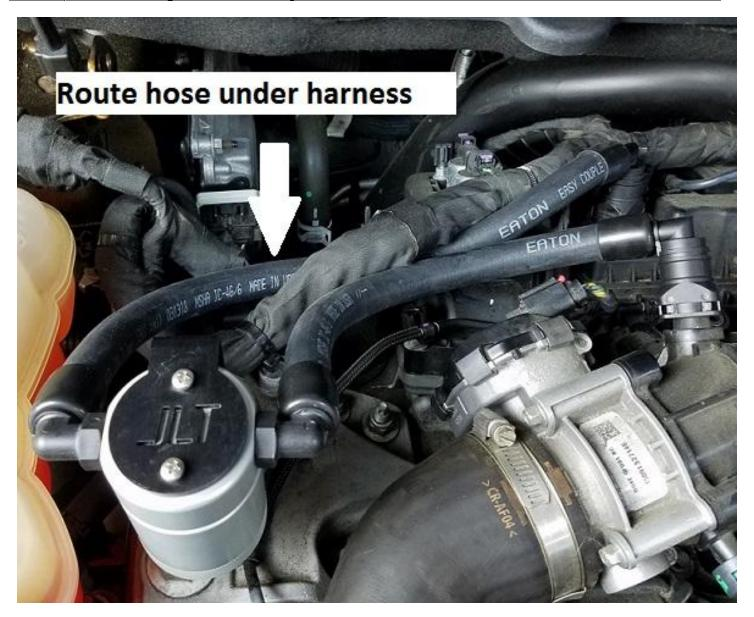
To properly clean the filter in the Oil Separator spray any degreaser or solvent through it and let it air dry. Clean it every 10,000 miles. Thanks for the business.
