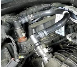
Locate 13mm bolt that holds a rubber isolator on the engine mount and remove bolt. Install JLT Bracket in the same location and reinstall bolt.
