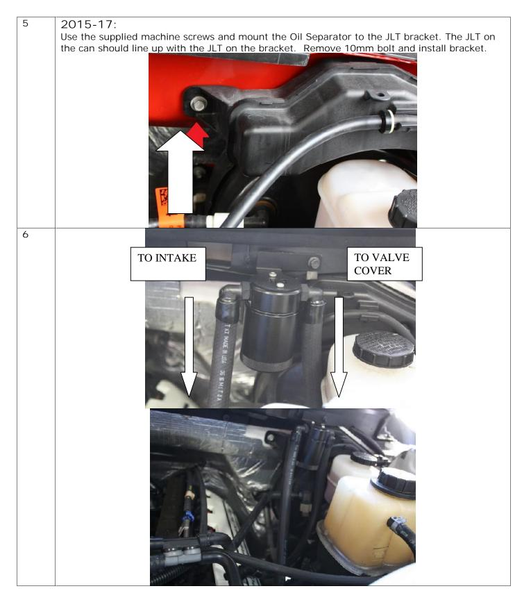
To properly clean the filter in the Oil Separator, remove the can from the truck and spray any degreaser or solvent through it and let it air dry. Clean it every 15,000 miles. Thanks for the business.
