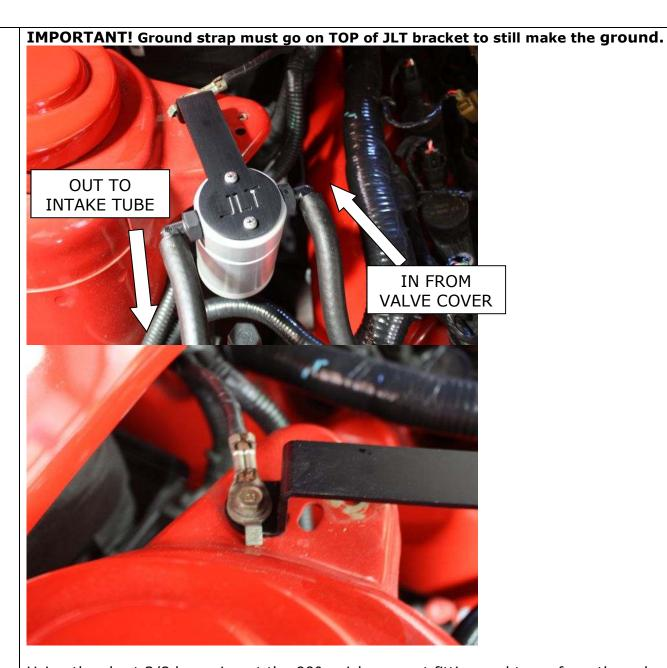
Using the short 3/8 hose, insert the  $90^{\circ}$  quick connect fitting and to go from the valve cover to the "T" side fitting on the Separator and the long 3/8 hose to go from the front most fitting to the intake tube.
