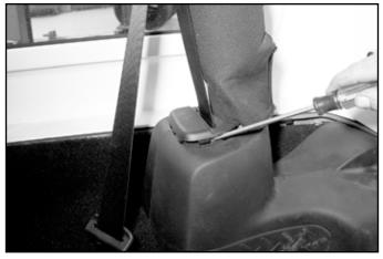
O Pull on the outside cover to release the clips and remove it.
