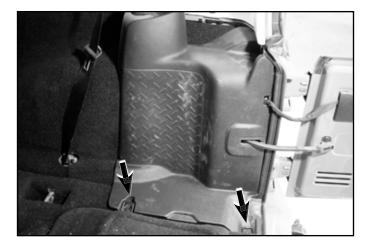
O Lastly, remove the nut located in front of seat belt to remove the inner plastic cover
