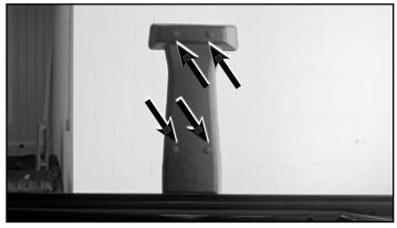
O Remove the spare tire mounting bracket from the tailgate by removing the 8 bolts using a 13mm socket.
