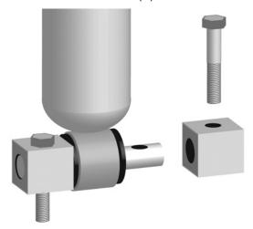
O Slide remaining Mounting Block (B) onto opposite end of Cross Pin (A).
